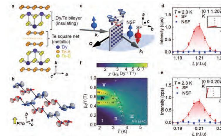
Non-coplanar helimagnetism in the layered van-der-Waals metal DyTe<sub>3</sub>. a, Crystallographic unit cell. b, Zigzag chain illustration of the non-coplanar magnetic ground state. c, Experimental geometry for polarized neutron scattering. d, e, Polarization analysis for the incommensurate cycloidal reflection. f, Magnetic phase diagram.
