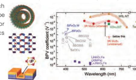
Left: Symmetry controlled TMDs. From the top, TMD nanotube, van der Waals heterostructure, and strained device. Copyright: Adapted from "Nature Nanotechnology 18, 36 (2023)." Right: Wave length dependence of bulk photovoltaic coefficient for nano TMDs.
