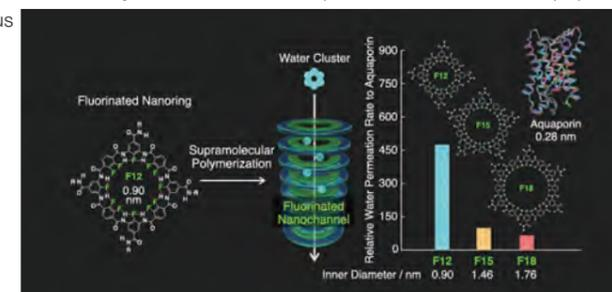
Fluorinated Nanotubes for Ultra-Fast Water Permeation and Their Inner Diameter Dependence
