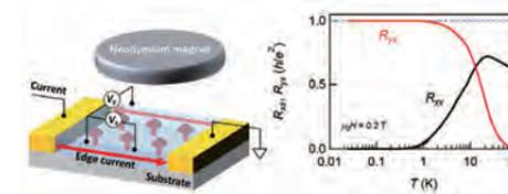
(Left) Schematic illustration of the quantum anomalous Hall effect device with a small permanent magnet. (Right) Temperature dependence of the longitudinal ( $R_{xx}$ ) and Hall ( $R_{xy}$ ) resistance.
