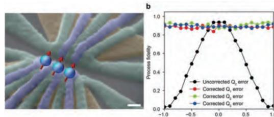
Figure (Left) Silicon three quantum bit device used for the experiment. (Right) Result of quantum phase error correction (Error recovery for the data qubit Q2).
