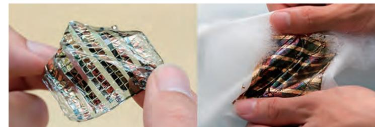
(Left) Ultraflexible organic solar cells manufactured on a 1 μm-thick plastic film.
