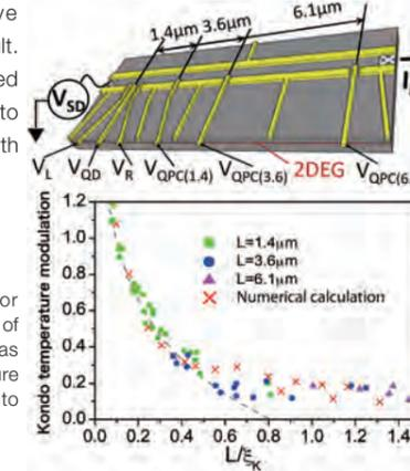
Schematic illustration of the device used for observation of the Kondo cloud and real shape of the Kondo cloud. The Kondo cloud shape was obtained by quantifying the Kondo temperature modulation by the gate voltage VQPC applied to the quantum point contacts.
