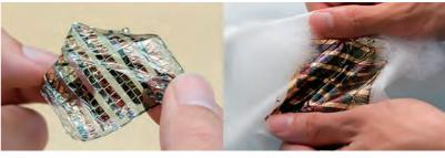
(Left) Ultraflexible organic solar cells manufactured on a 1 um-thick plastic film. (Right) Photograph of the washing process for the devices conforming to a dress shirt.
